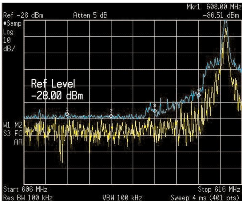
**Figure 1.** This over-the-air spectrogram shows signals from the Boston TV38 station (the peak on the right) extending down into the UHF WMTS band. The signals between diamond-shaped markers 3 and 4 (612 and 614 MHz, respectively) are from the TV station and are legal even though they prevent use of this segment of the WMTS band. The bottom trace is real-time and the top trace is max hold.
