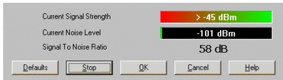
Figure 4.1 – SNR as reported by Cisco’s Aironet Client Utility.
