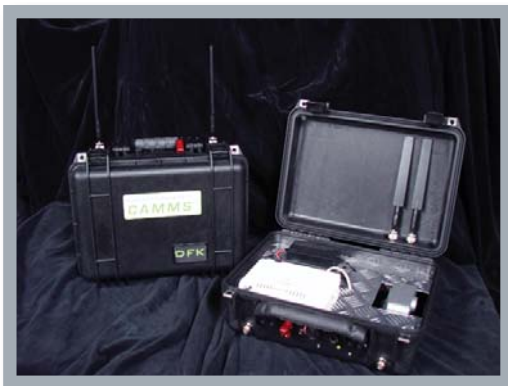
CAMMS™ DFK-RC interior with AP, camera & battery
