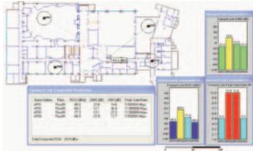
Simulate a mobile client in a GSM network
